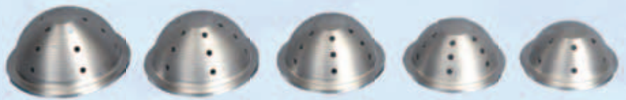
Impactor head sizes of \varnothing 42 , \varnothing 46 , \varnothing 50 , \varnothing 54 and \varnothing 58 mm
